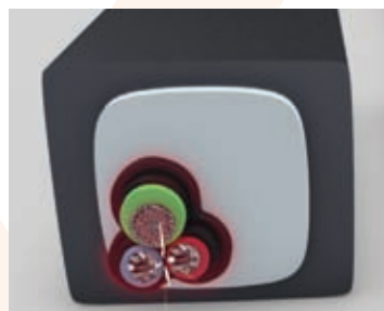
Sectional view of other company's heating cable
